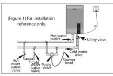
Installation must be made by installers of or designated by our company after-service department. The water heater shall be wall-mounted.
